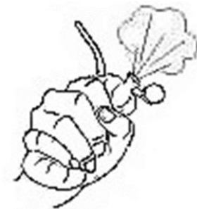
Squeeze the bulb flat with your hand before you replace the plug.
