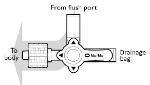
In this drawing, the stopcock switch points to the drainage bag. (The word "OFF" is closest to the drainage bag.) This position allows you to inject fluid into the tube from the flush port.
