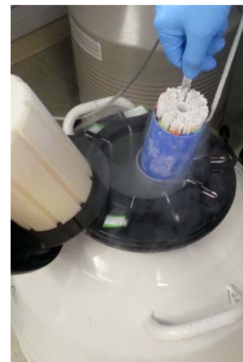
Large tanks filled with liquid nitrogen keep sperm frozen and safe for at least 75 years.
